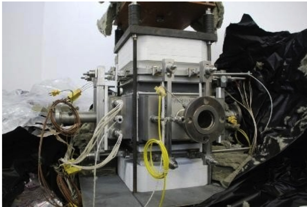
Fig. 39 – 1 kW MCFC stack, Warsaw University of Technology.
