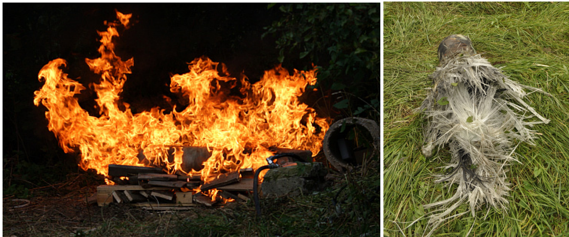
Fig. 8. The bonfire test of high pressure vessel and view of the vessel after this test if PRD failed.
