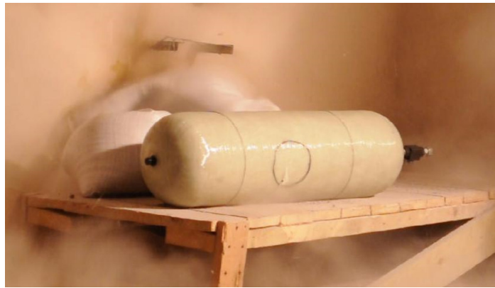
Fig. 7. High pressure vessel during the penetration test.
