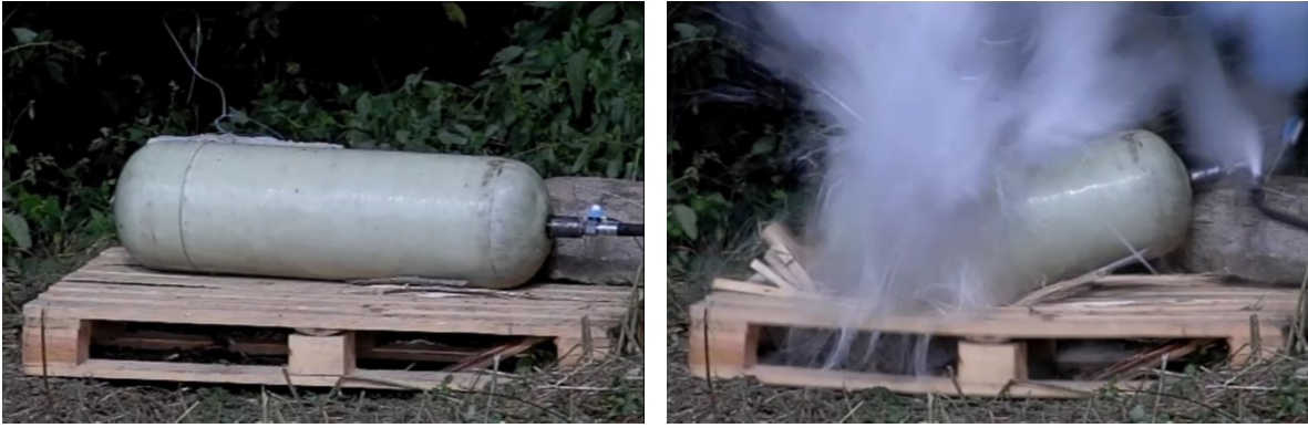
Fig. 6. Burst test of high pressure vessel in the test range conditions.
